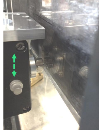
Fig. 2. Set-up for parametric study investigating the influence of different geometries of permanent magnet systems on the Lorentz force. Their volume ( 1000 \text{ mm}^3 ) and the flow rate ( Re \approx 7000 ) of GaInSn are held constant. On the figure the magnet is placed in y = -25 \text{ mm} and moves vertically (double sided arrow) until reaching the top wall of the duct ( y = 25 \text{ mm} ).
